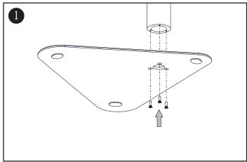
1. Mount the counter top with (3) M5x16 counter sunk screws to the base plate or on the existing table area.
