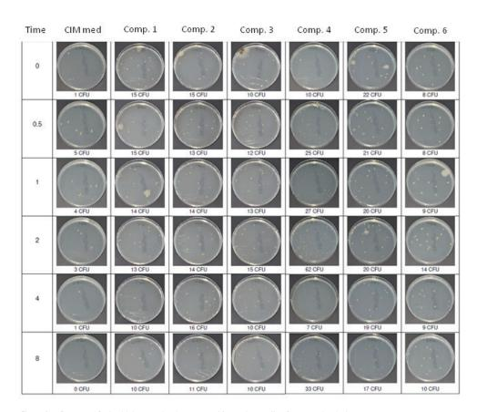
Figure 1: Summary of microbial contamination recovered by swab sampling from complex design structures (hinges, cable duct inlets and outlets, gaps and any other uneven surfaces).
